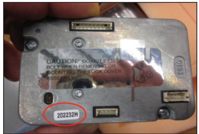
The lock body has label 202232H on case cover, which denotes the Gen2 firmware upgrade level to 2.0.929.
