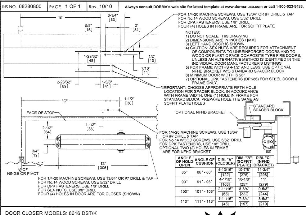
DOOR CLOSER MODELS: 8616 DS1/K DOOR SAVER (PARALLEL ARM MOUNT) FOR USE WITH STANDARD SPACER BLOCK FOR USE WITH OPTIONAL NFHD BRACKET
