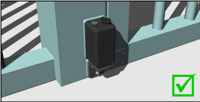
Lock mounted to the gate frame vertically down.
