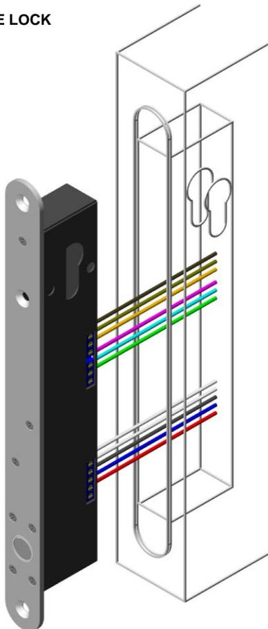
The wiring options and detail is shown overleaf. Once the desired wiring method is chosen run the wires into the rear of the mortice and connect to the lock. There are screw terminals for each wire and a connector guide is shown on the lock cover.
