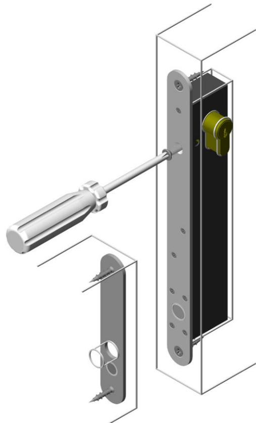
Slide the lock back into the mortice, making sure that the wiring integrity is maintained. Secure the lock and strike plate in place, using the supplied mounting screws. Fit the euro profile cylinder into the lock and secure in place with the M5 screw provided. Ensure that the hole behind the strike plate is free from swarf and is deep enough to allow the lock pin to fully extend when locked.
