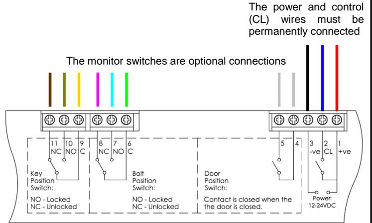
In either fail safe or fail secure configuration, maintained connection of '1' to '2' will keep the DB25K unlocked regardless of door position.
