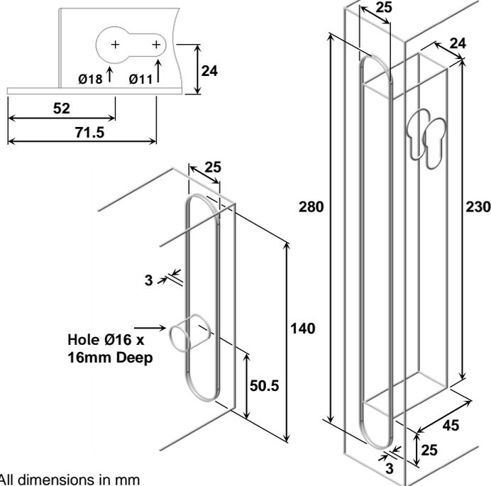
Cut mortices into the door and door frame for the strike plate and lock as per the dimensions shown. In addition a hole is required through either one or both sides of the mortice to allow a euro profile cylinder to be fitted. The top end of the strike plate must be aligned with the top of the lock so the bolt pin goes centrally into the hole in the strike plate. The gap between the lock face plate and strike plate must not exceed 6mm when the door is closed.
