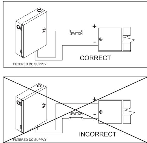
**Fig. 2 – Power Connections**
