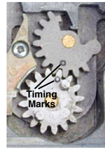
Figure 6 - Do Not Remove Metal Gears
