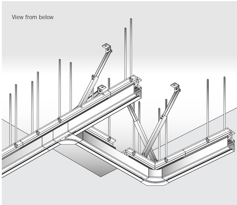
The construction of the stacking area, assembled from substructure and track rail modules, provides a good illustration of how this well-designed system can be utilised. The individual components are coordinated to ensure safe integration. Joints in the substructure are offset to those in the track rails so that individual joints coincide with continuous material in all cases.
