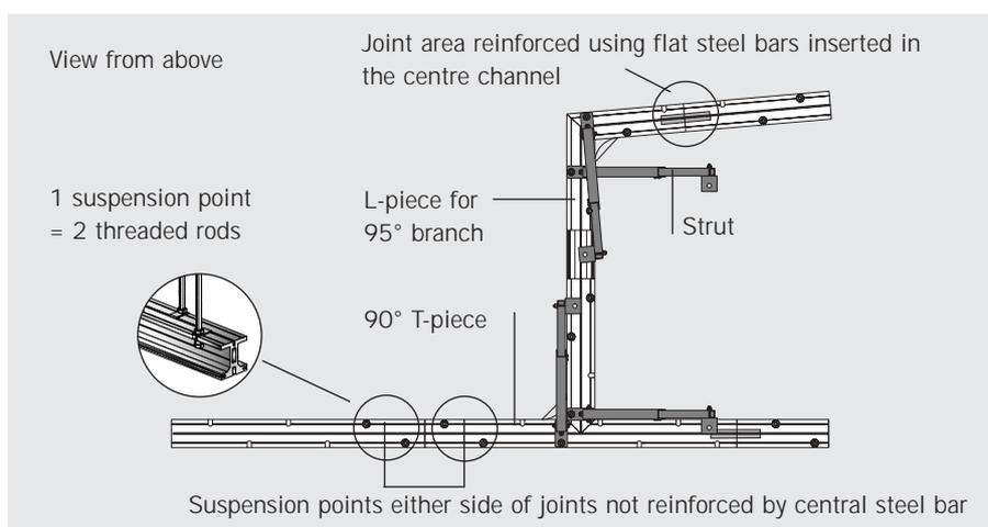
Joints reinforced by central steel bar only require one local suspension point.
